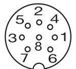
Fig. 4-2: Pin assignments BKS, connector type BTL
